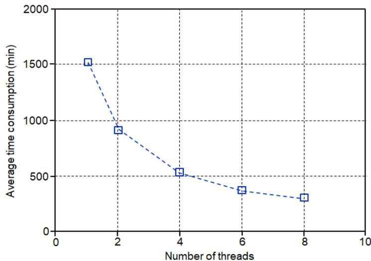
Figure 17: Relationship between average computing time and thread number in 3D SPH modelling.
