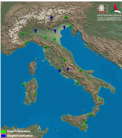
1057 Figure 13: The radar network of the Department of Civil Protection. Green radars operate with dual-polarisation, blue 1058 radars have single polarisation.
