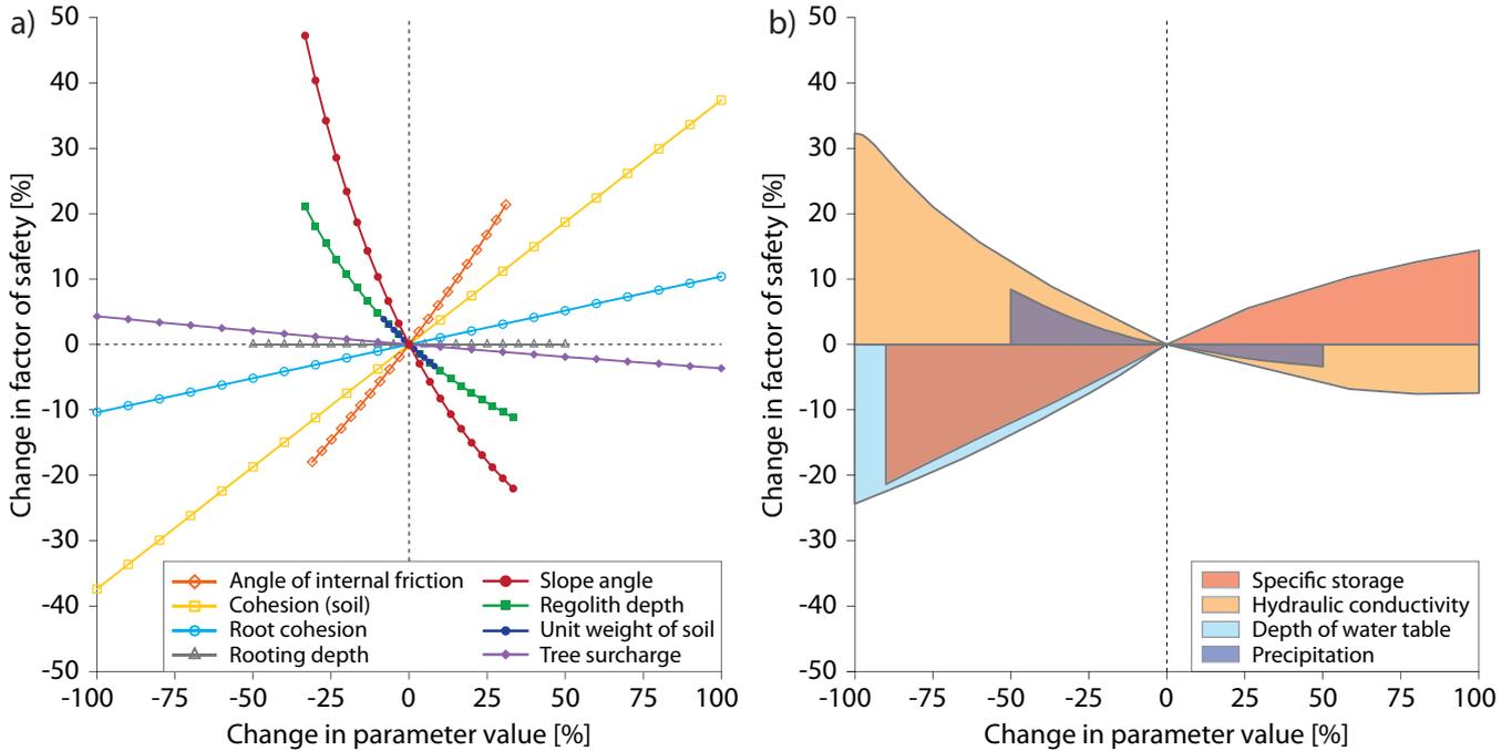
**Figure 8.** OAT sensitivity of the model results (change in factor of safety) for tested parameter value ranges for the geomechanical model element (a) and the hydrological model element (b). Respective parameter values are listed in Table 4.
