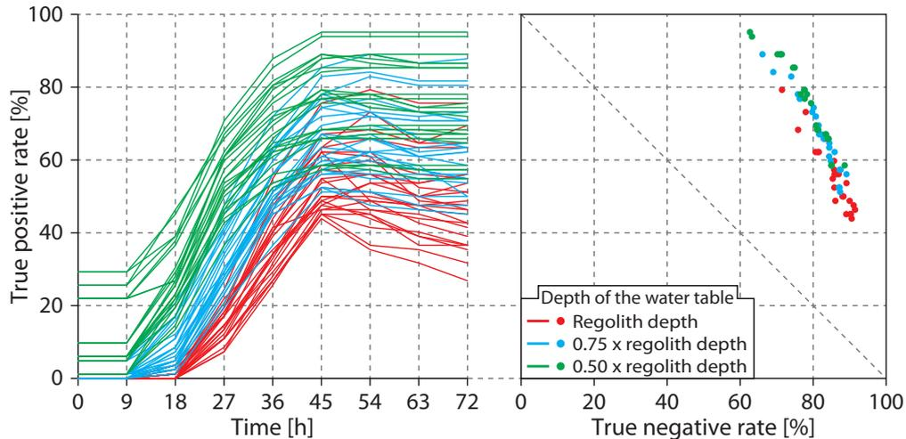
**Figure 10.** Temporal prediction rate (a) and coordinates for  $FOS=0.99$  and  $FOS$  falling below 1.0, based on the model ensemble for the landslide-triggering rainfall event in May 1999. Three scenarios for the initial conditions (initial depth of the water table) are considered.
