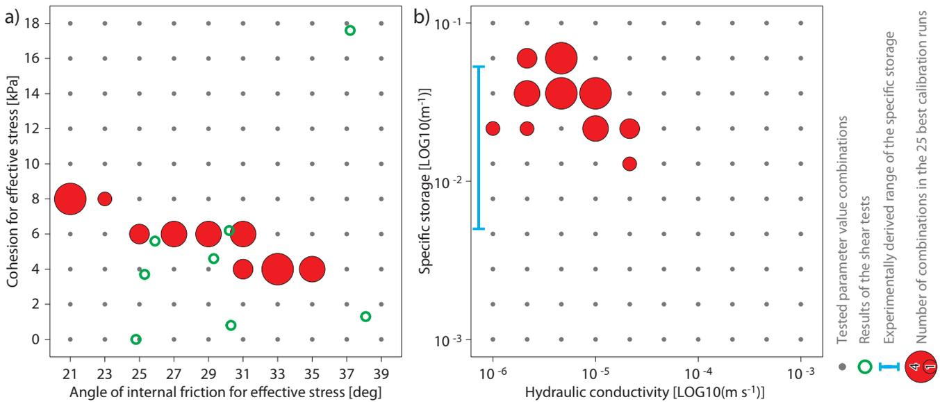
**Figure 12.** Calibrated values for the geotechnical (a) and hydrological parameters (b). The sizes of the red circles indicate the number of model runs based on these value pairs (with varying values of the further tested parameters). The results of the shear tests are shown in (a) as green circles. The experimentally derived range of the specific storage is indicated by the blue bar in (b).
