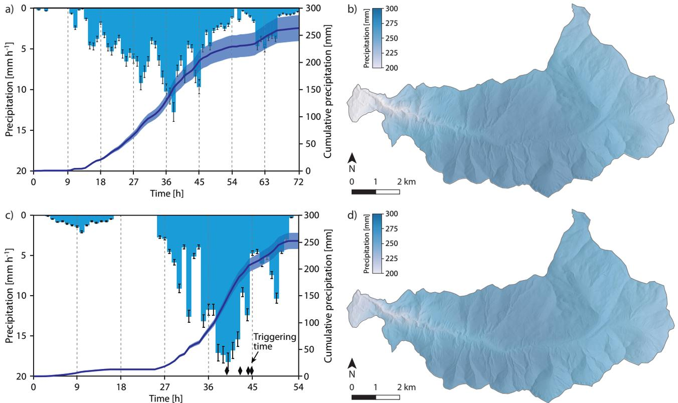
**Figure 4.** Hourly precipitation time series (a, c) and spatially interpolated precipitation sums (b,d) for the duration of the landslide-triggering rainfall events in 1999 (a,b; 20 May, 07:00–23 May, 07:00) and 2005 (c,d; August 21, 07:00–August 23, 12:00). The error bars and the shading for the cumulative precipitation sum in (a) and (c) indicate the range of the interpolated hourly precipitation sums within the catchment area.
