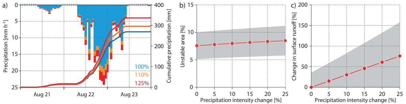
**Figure 13.** Scaled rainfall event of August 2005 (a) and resulting changes in slope stability (b) and surface runoff (c), based on the ensemble runs with a scaled precipitation input (b). The area shaded in grey shows one standard deviation.
