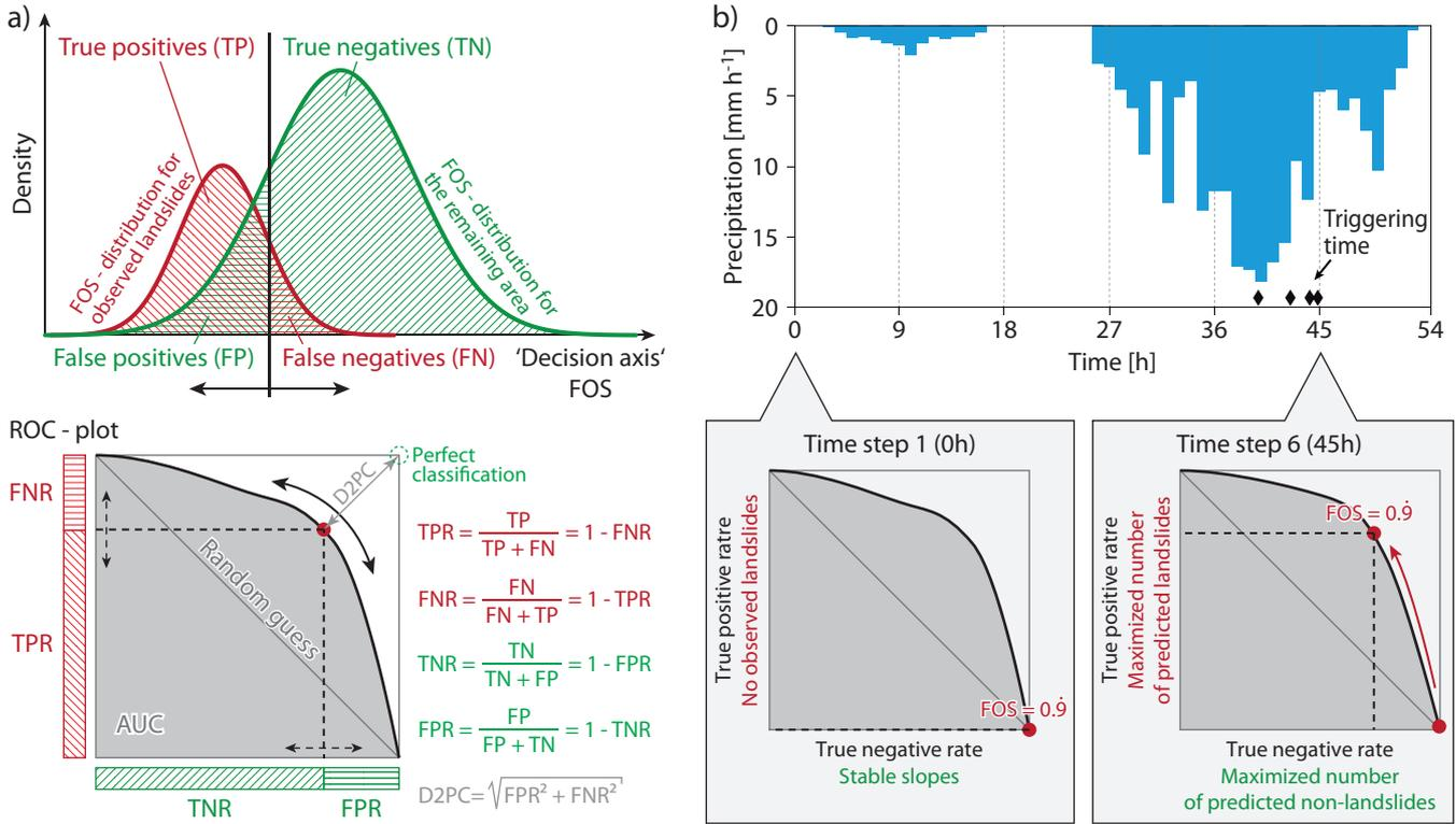
**Figure 7.** Principle of the receiver operating characteristic (a; modified after Metz, 1978) and its application in the calibration procedure (b). FOS: factor of safety, TPR: true positives rate, FNR: false negatives rate, TNR: true negatives rate, FPR: false positives rate, D2PC: distance to perfect classification, AUC: area under the ROC-curve.
