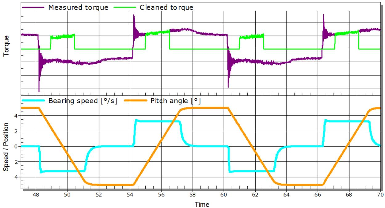
**Figure 3: Oscillating rotations and torque measurements (example)**
