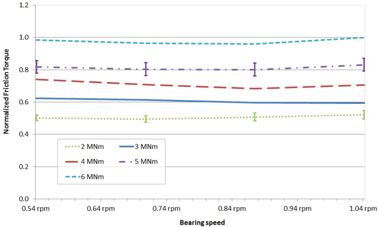
**Figure 6: Measured friction torque at different speeds and loads**
