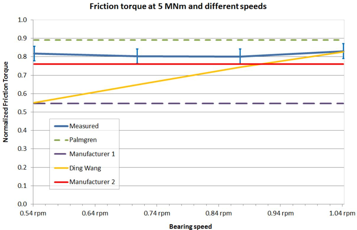
15 Figure 8: Measured and calculated friction torque at different speeds and 5 MNm load
