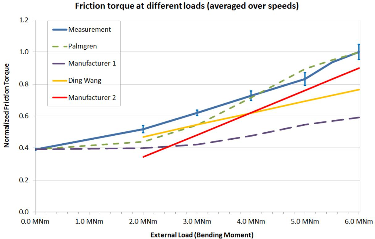
5 **Figure 7: Measured and calculated friction torque at different loads**
