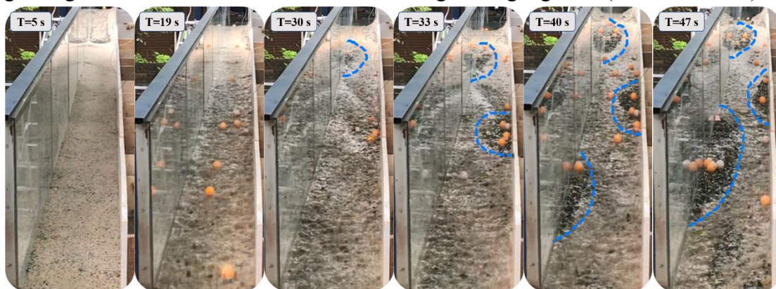
Figure. 3 The riverbed morphology at six different moments during the boulder bars' formations and growths process for the T7 experiment. The boulder bars in the figure are marked with blue dotted lines.
