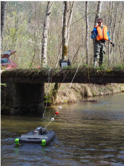
Figure 3: (a) Drifting board sharing the hydrophone and the acoustic recorder; (b) Drift trajectories of the recorder during the measurements.
