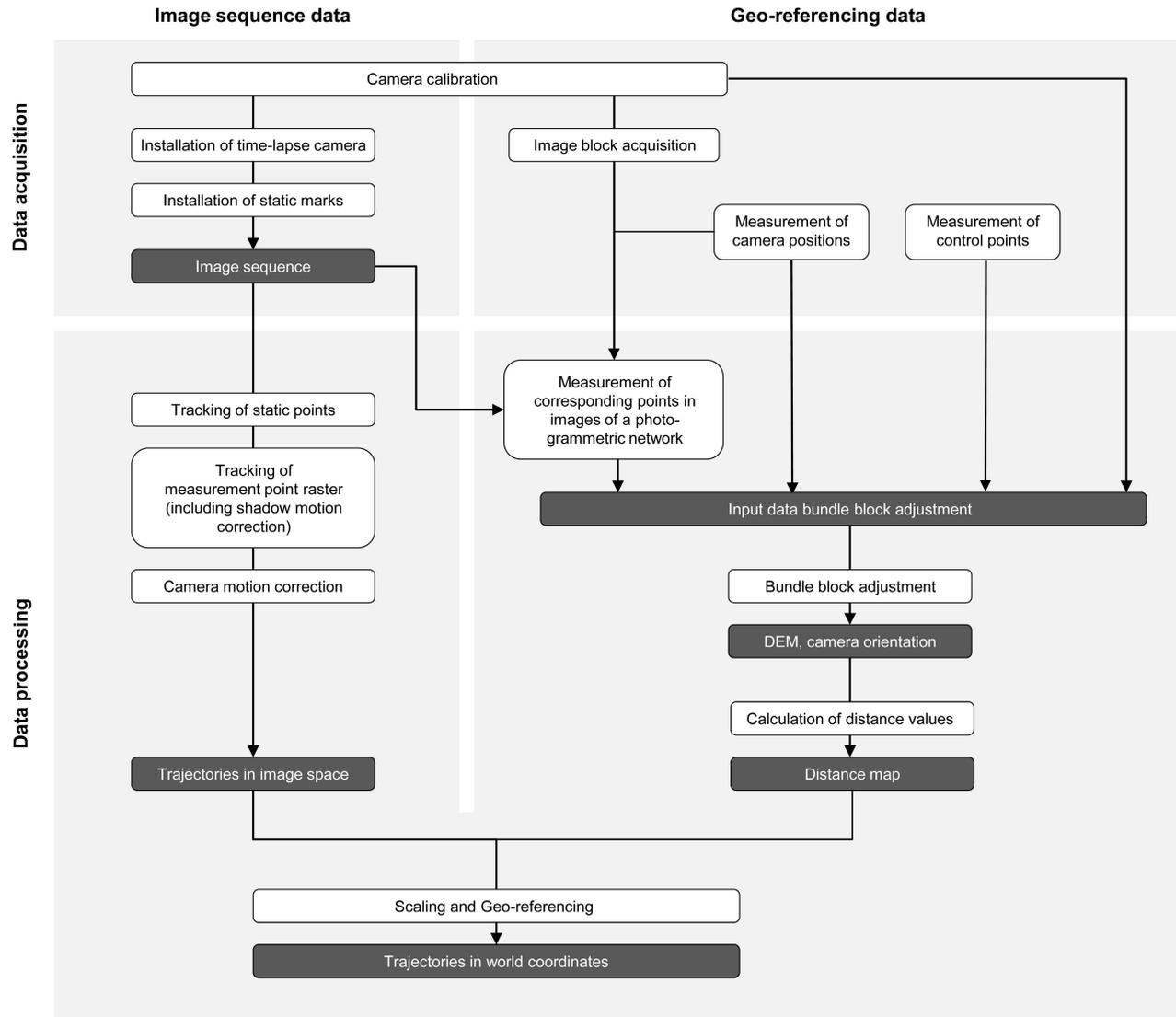
Figure 2: Workflow of monoscopic image sequence measurement
