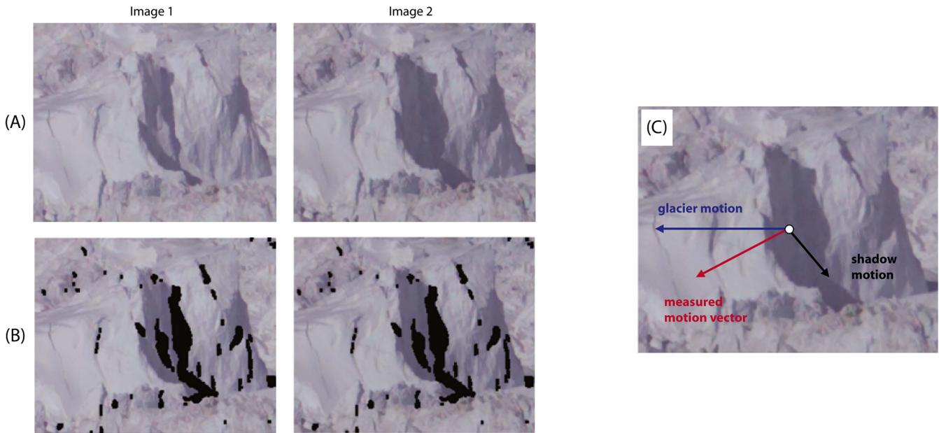
**Figure 6: Influence of moving shadows in image sequences. The figure shows corresponding image sections from two sequence images recorded at a time interval of 30 min (A). In the same image pair those pixels were marked black, which are influenced by shadow motion (B). These pixels falsify the result of the feature tracking because the tracked glacier movement is overlaid by the shadow movement (C).**
