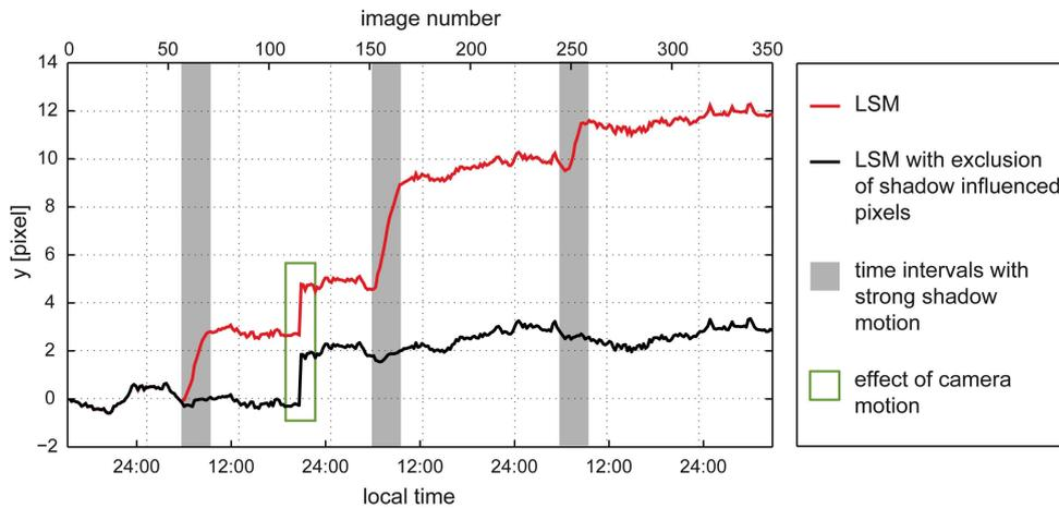
5 | **Figure 8: Drift effects during the measurement of a trajectory due to shadow movement. The figure shows the vertical component of a glacier trajectory measured using least squares matching (LSM) with and without shadow pixel exclusion. At certain times of the day (gray background) particularly strong shadows occur. Both motion curves still contain the influence of the camera motion.**
