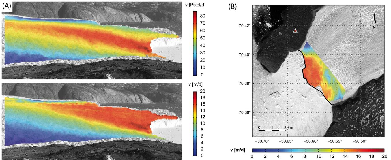
**Figure 11: Result of scaling (A) and geo-referencing (B) at Støre Qarajaq glacier. The figure shows the color-coded superposition of velocity values derived from measured trajectories. They are shown as unscaled values in image space (A, top) and scaled values transferred into object space (A, bottom), as well as geo-referenced values that can be overlaid on satellite images (B).**
