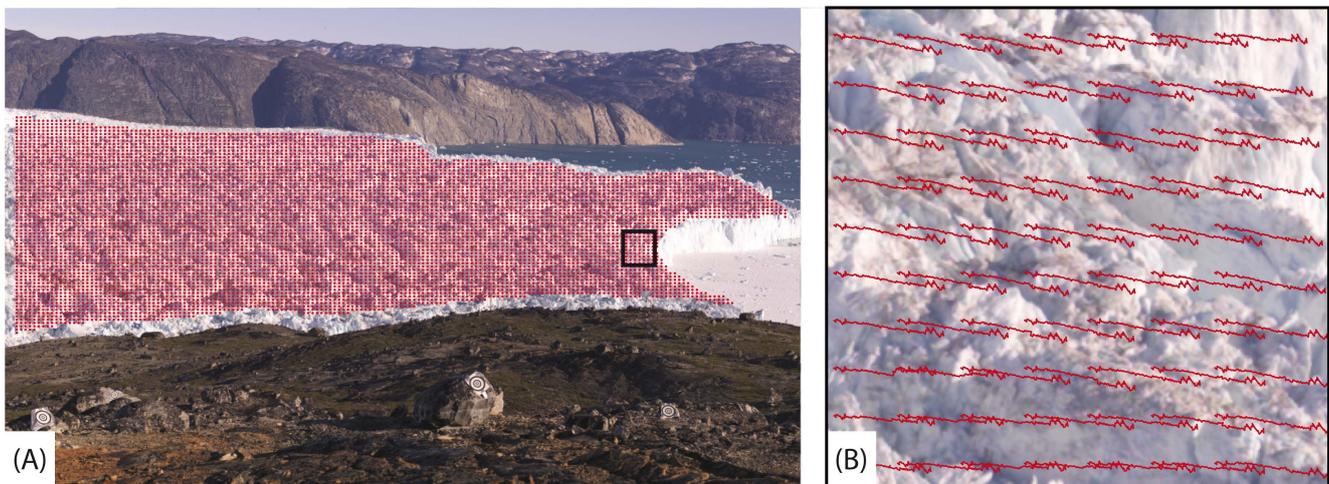
25 **Figure 5: Raster of measurement points on the glacier surface (A) and resulting trajectories obtained from feature tracking (B). The figure shows the grid of the measuring points (red dots) as a superposition of a sequence image (A). For the black-marked area, the corresponding image section is shown on the right. It is superimposed by the measured trajectories (red lines) for a 24 h image sequence (acquisition interval 20 min) (B).**
