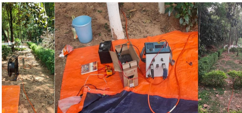
Figure.4: SYSCAL Pro-96 (Iris Instrument) data-acquisition field setup using 96 electrodes
