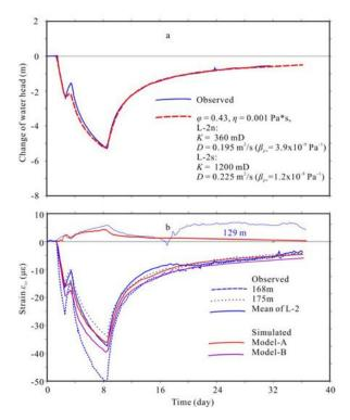
Figure 1. Observed and simulated (a) water head and (b) vertical strain (zzz) in Lei et al. (2019)
