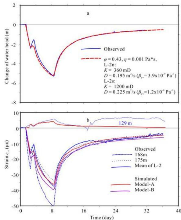
Figure 1. Observed and simulated (a) water head and (b) vertical strain ( $\epsilon_{zz}$ ) in Lei et al. (2019)
