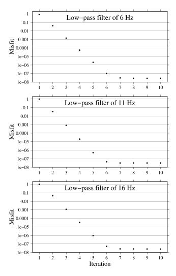
**Figure 12.** Misfit decrease plotted in a log axis along the iterations. The upper panel corresponds to the misfit reduction of the seismic information contained in the first multi-scaling step (low-pass filter of 6 Hz), the middle one for an intermediate step (low-pass filter of 11 Hz), and the lower panel for the final frequency band inverted (low-pass filter of 16 Hz).
