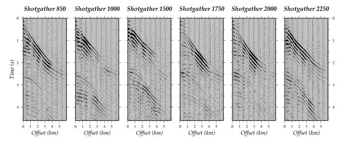
Figure 6. Seismic data obtained from the DC of the streamer shots recorded in the TOPOMED cruise, only 16 traces each km are plotted.
