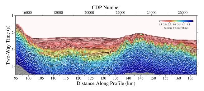
**Figure 13.** Two-way-time transformed VP model obtained after the modeling sequence proposed on this paper (joint DC refraction and streamer reflection TTT + FWI) is shown superimposed to the time migrated MCS image.
