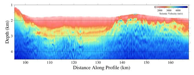
Figure 10. Final velocity model after the FWI using Fig. 7d as initial model.
