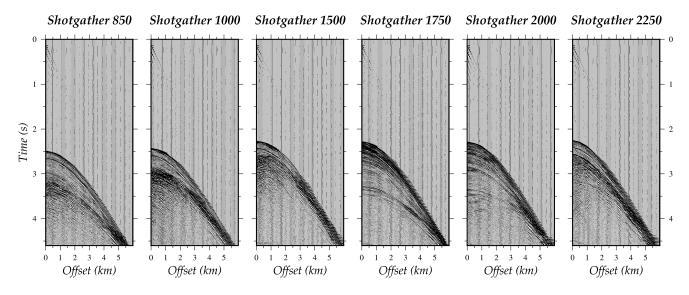
Figure 4. Decimated example of the field data set, only 10 traces each km are plotted.
