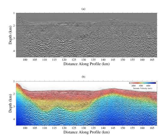
Figure 14. a) Kirchhoff depth migration result based on the velocity model shown below (b) obtained after the joint DC refraction and sweamer reflection TTT.
