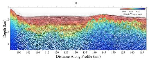
e 15. (a) Kirchhoff depth migration result based on the velocity model shown below (b) obtained after the modeling sequence proposed on this paper (joint DC refraction and streamer reflection TTT + FWI).
