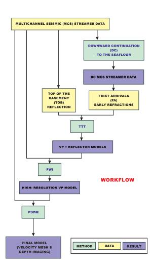
Figure 1. General scheme of the workflow. We build the  $V_P$  model sequentially, from long- to small-scales, taking advantage of all the information contained in our data. We apply the different techniques referred in the text (DC + TTT + FWI + PSDM) to obtain a high-resolution image of the subsurface.
