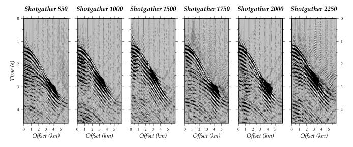
**Figure 5.** Seismic data obtained after the first DC step of the streamer shots recorded in the TOPOMED cruise. The wavefield are displayed for every fifth trace.
