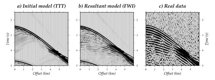
**Figure 11.** Streamer synthetic seismograms, which are computed using the initial and final velocity model presented in Fig. 7d and Fig. 10 and the FD solver of the FWI algorithm, together with the observed shotgather. The field seismogram is displayed for a better comparison of the results. The location of the streamer is at a distance of 101 to 107 km along profile. Only one trace every 50 m is plotted.
