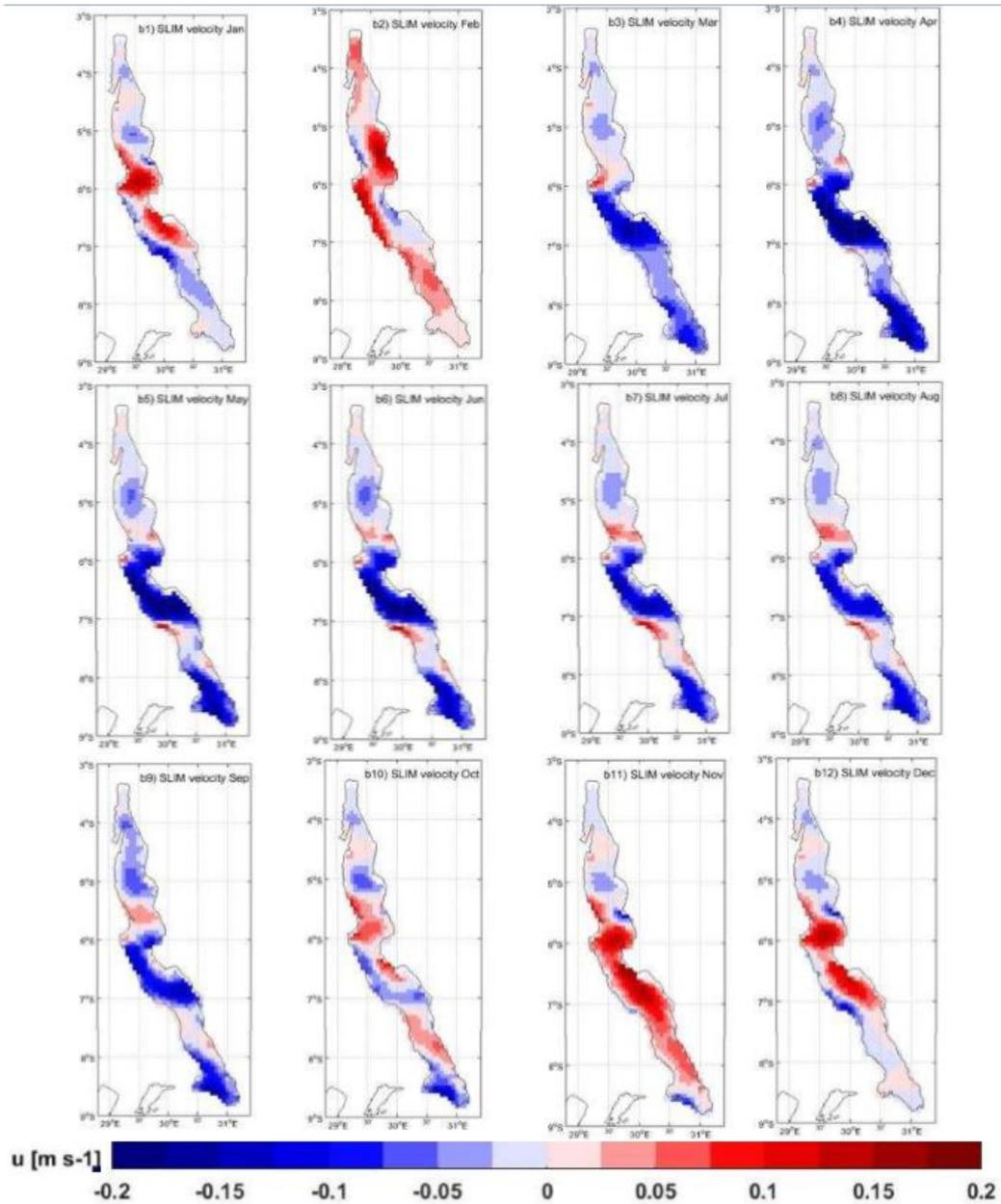
**Illustration 4: Monthly average surface water velocity obtained from the EVAL simulation with positive (red) values showing northbound displacement and negative (blue) values showing southbound displacement.**
