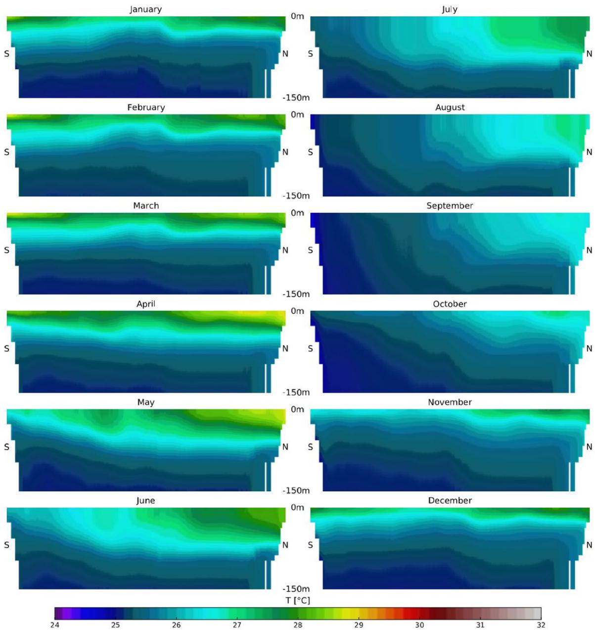
**Fig. 9: Monthly water temperature cross-sections (as defined in Fig. 1b) obtained by the HIS-simulation.**
