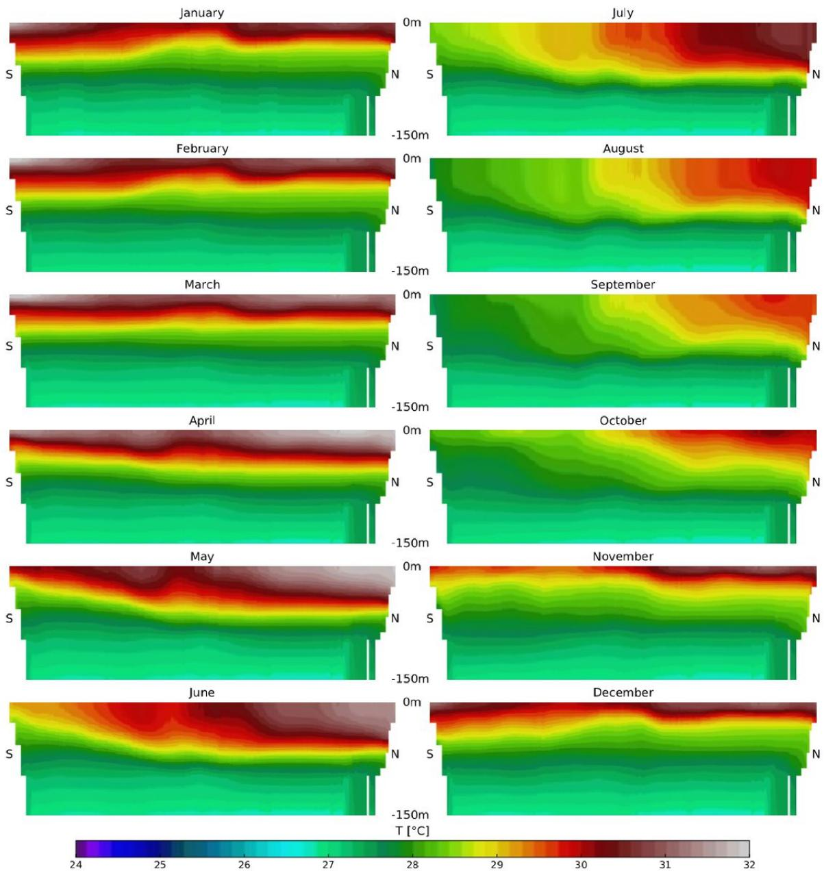
**Fig. 10: Monthly water temperature cross-sections (as defined in Fig. 1b) obtained by the FUT-simulation.**
