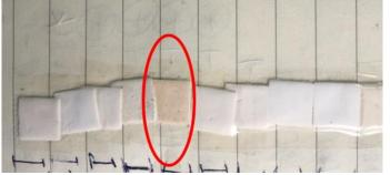
**Figure R1.** A photo of filters after OC/EC analysis. The red circle highlights an example of abundant metal oxides on the quartz filter after OC/EC analysis, leading to browning of the filter.
