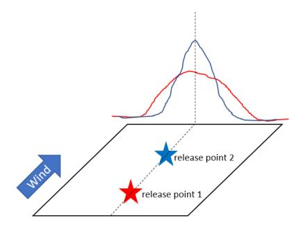
In this case any release location along the dotted line will result in the same modelled plume-centre location. But a source at release point 2 with a low emission rate will produce the same plume amplitude as a source at release point 1 with a high emission rate. These would produce the same value of J for this transect.
