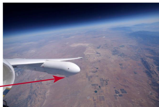
Figure 1. (a) Cross-section image of AirHARP instrument rendered using CAD software; (b) AirHARP instrument mounted on ER-2 aircraft left-wing front pod (Image courtesy: Brent McBride); (c) Image captured by NASA Science Pilot D. Stuart Broce, during the ACEPOL flight on Oct-26 2017. The red arrow in the figure points to the AirHARP's exposed part when mounted on the wing pod.
