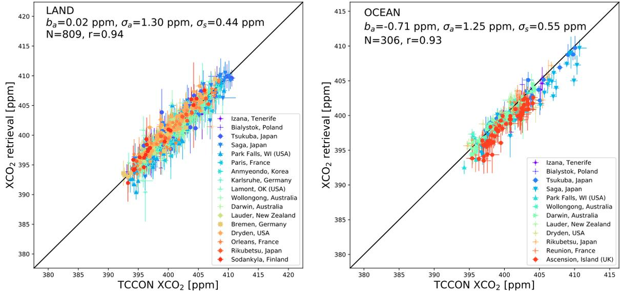
**Figure 1.** XCO<sub>2</sub> retrievals by using only the 2.06  $\mu\text{m}$  band of OCO-2. We evaluate overpass averaged results over land and ocean separately. In each panel, we include bias ( $b_a$ ), standard deviation of the difference ( $\sigma_a$ ), station-to-station variability ( $\sigma_s$ ), number of overpass (N), Pearson correlation coefficient ( $r$ ) and one-to-one line. For each overpass, variations of XCO<sub>2</sub> retrievals and TCCON data are presented with errorbars.
