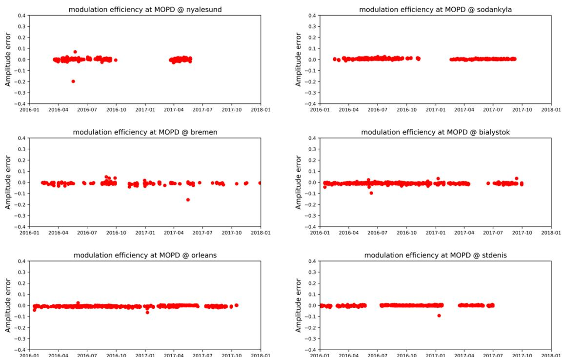
Figure 1. the time series of the retrieved amplitude of the modulation efficiency at maximum path difference (45 cm) at six sites.
