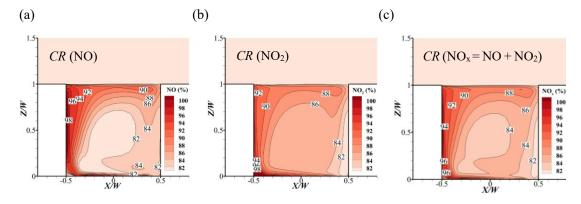
The change rate of NO, NO2 and NOx between different ventilation conditions
