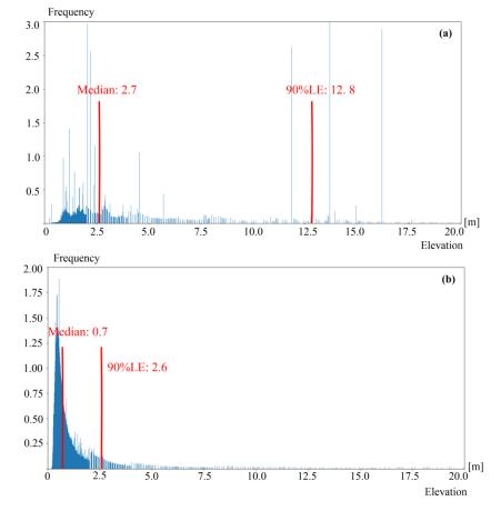
Figure R4 Histograms of random elevation errors of (a) REMA mosaic and (b) TDM DEM covering AP. Median value and 90% quantile of the errors (90%LE) are marked in red in the histograms.
