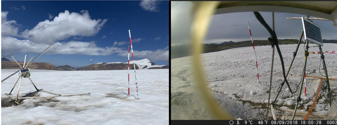
**Figure 2** Left side photo shows hunting-camera and mass balance stakes close to top of the August-one ice cap, right side photo showed hunting camera photographed rough ice surface on September 8 of 2018 and ice surface stake gauge at the automatic photogrammetry site.
