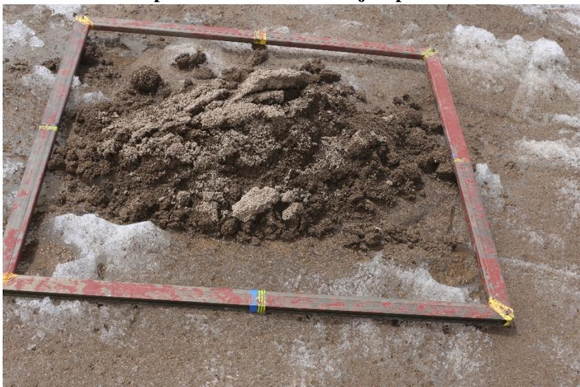
**Figure 3** Aluminum frame used as control field for Geo-referece at August-one ice cap. The hummocky is covered by cryoconites (grey part is sun dried cryoconite, brown part is wet cryoconite).
