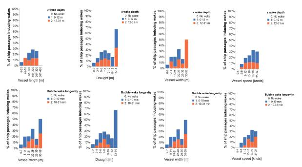
Figure 6. Example figures of how the vessel length, draught, width and speed relates to the  $\varepsilon$  maximum wake depth and bubble wake longevity, for all single passages in the dataset. Note that for all parameters but vessel speed, the categories with the highest values (rightmost bars) have very few passages (<10).
