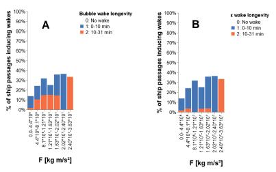
Figure 4. Wake longevity in minutes for the bubble wake (a) and dissipation rate of turbulent kinetic energy ( $\varepsilon$ ) wake (b), for all single passages. The x-axis shows the force (F) of the vessel in Newton, calculated as seawater density\*ship width\*ship draught\*ship speed². Wake temporal longevities < 10 min are shown in blue and wake longevities 10–30 min are shown in orange.
