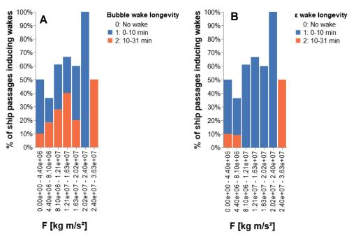
Figure 3. Wake longevity in minutes for the bubble wake (a) and dissipation rate of turbulent kinetic energy ( $\varepsilon$ ) wake (b), for the wakes induced by ships passing at 0-3 ship widths from the instrument. The x-axis shows the force (F) of the vessel in Newton, calculated as seawater density\*ship width\*ship draught\*ship speed². Wake temporal longevities < 10 min are shown in blue and wake longevities 10–30 min are shown in orange.
