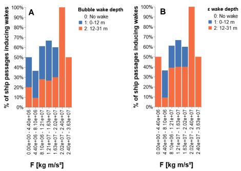
Figure 1. Maximum wake depth for the bubble wake (a) and dissipation rate of turbulent kinetic energy ( $\varepsilon$ ) wake (b), for the wakes induced by ships passing at 0-3 ship widths from the instrument. The x-axis shows the force (F) of the vessel in Newton, calculated as  $\rho$ \*ship width\*ship draught\*ship speed². Wake depths within the range presented in previous studies are shown in blue and wakes deeper than previously reported are shown in orange.
