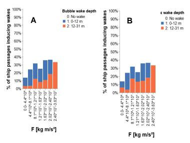
Figure 2. Maximum wake depth for the bubble wake (a) and dissipation rate of turbulent kinetic energy ( $\epsilon$ ) wake (b), for all single passages. The x-axis shows the force (F) of the vessel in Newton, calculated as seawater density\*ship width\*ship draught\*ship speed². Wake depths within the range presented in previous studies are shown in blue and wakes deeper than previously reported are shown in orange.
