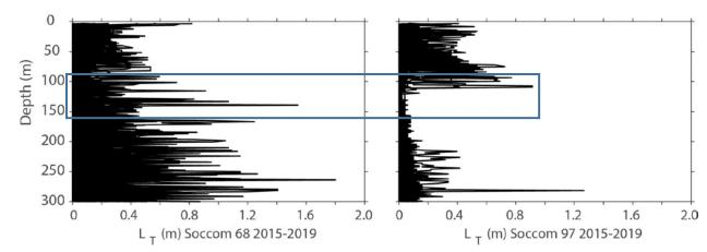
Figure 1. Thorpe scale, float \*68 (over Maud Rise) and \*97 (North of Maud Rise). (Blue rectangle) Note the remarkable decrease at the thermal barrier depth for float \*97 compared to the overturning at Maud Rise. Figure to be included in the manuscript as part of Figure 3.
