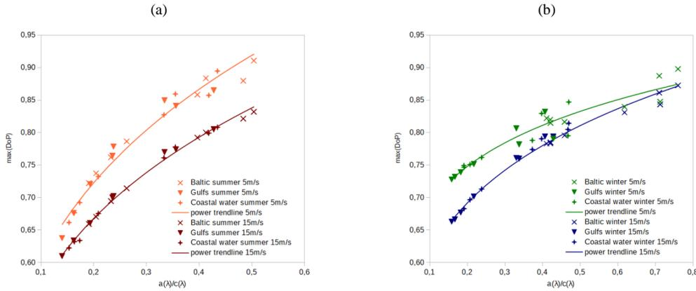
**Figure 7. Values of maximum of degree of polarization against absorption to attenuation ratios  $a(\lambda)/c(\lambda)$  for average values of IOPs presented in Table 1, plotted for (a) the summer season and (b) the winter season.**
