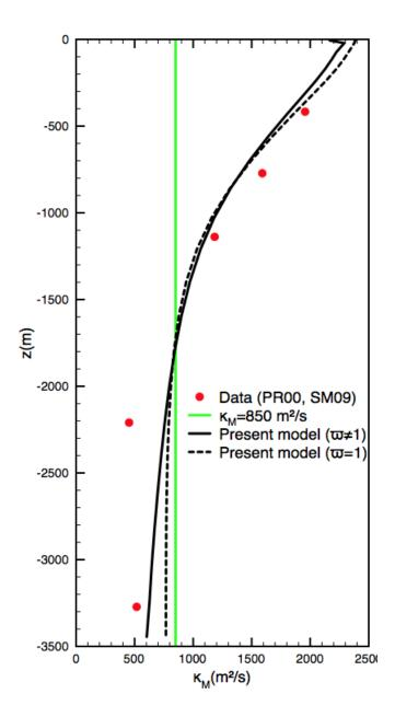
**Fig.3** Borrowed from Canuto et al. (2017b). Comparison of mesoscale diffusivity (in m<sup>2</sup>s<sup>-1</sup>) computed within D3 and CD5 model vs. the measured data of Philips and Rintoul (2000, PR00) in the ACC (143E, 51S). The  $\varpi = 1$  case is with the contribution of corrections of the higher order in the small parameter equal to the ratio (mean K/EKE).
