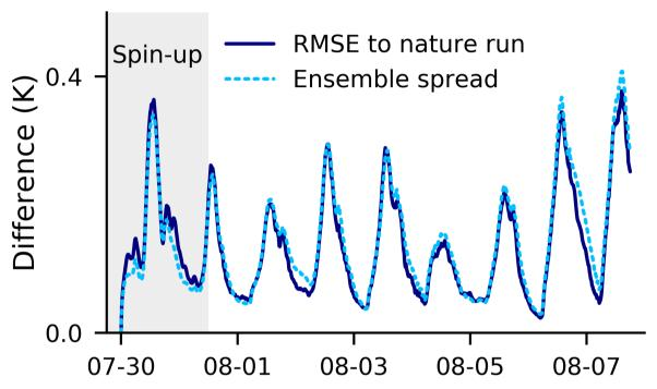
Figure 1: The spatially-averaged RMSE of the ensemble mean to the nature run and spatially-averaged standard deviation within the open-loop ensemble for the temperature in COSMO at 10 meters height.
