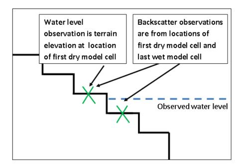
Caption: Figure 5: Schematic of observation locations used in this study for each transect in cross section. The thick black line shows the discretised domain elevation, the dashed blue line shows the observed flood water level. The arrows and green crosses show the locations of the observations.
