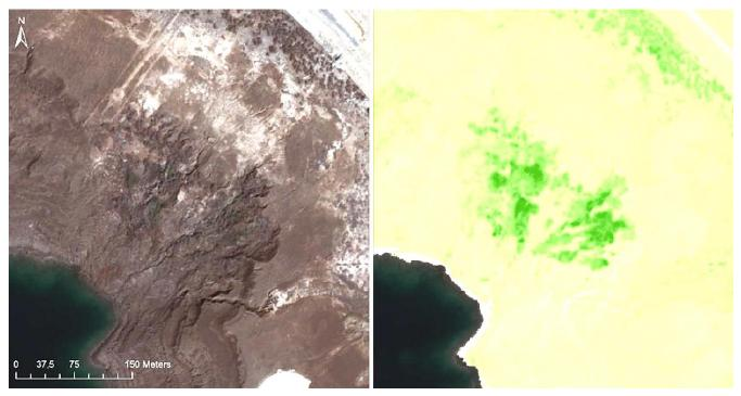
Figure 5: comparison between optical and NDVI image. Left: optical image (RGB) shows a seepage area. The muddy sediments impregnated with water and salt (white patches) flowed towards the lake and created an amphitheatre. This seepage zone has grown over time. Right: in this environment fill up with salt the vegetation (green) manages to develop only near the springs.
