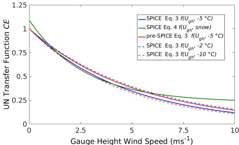
**Figure B1.** Transfer functions describing the unshielded (UN) catch efficiency (CE) as a function of the gauge height wind speed ( $U_{gh}$ ). The Eq. 3 results were produced by modelling CE with respect to wind speed at  $T_{air} = -5$  °C, and both the Kochendorfer et
