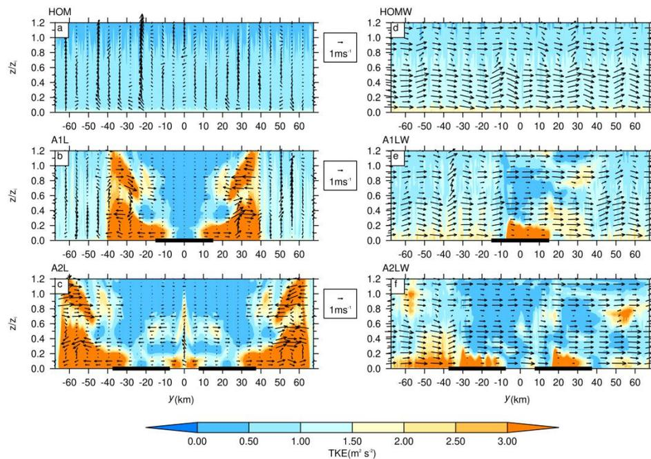
Fig. 6. The y-z cross sections of the TKE (contour) with superimposed wind vectors composed of  $v$  and  $w$  wind over (a, d) homogeneously heated and (b, e and c, f) heterogeneously heated surfaces with (d, e, f) and without (a, b, c) background flow. The black lines on the x-axis represent the lake patches.
