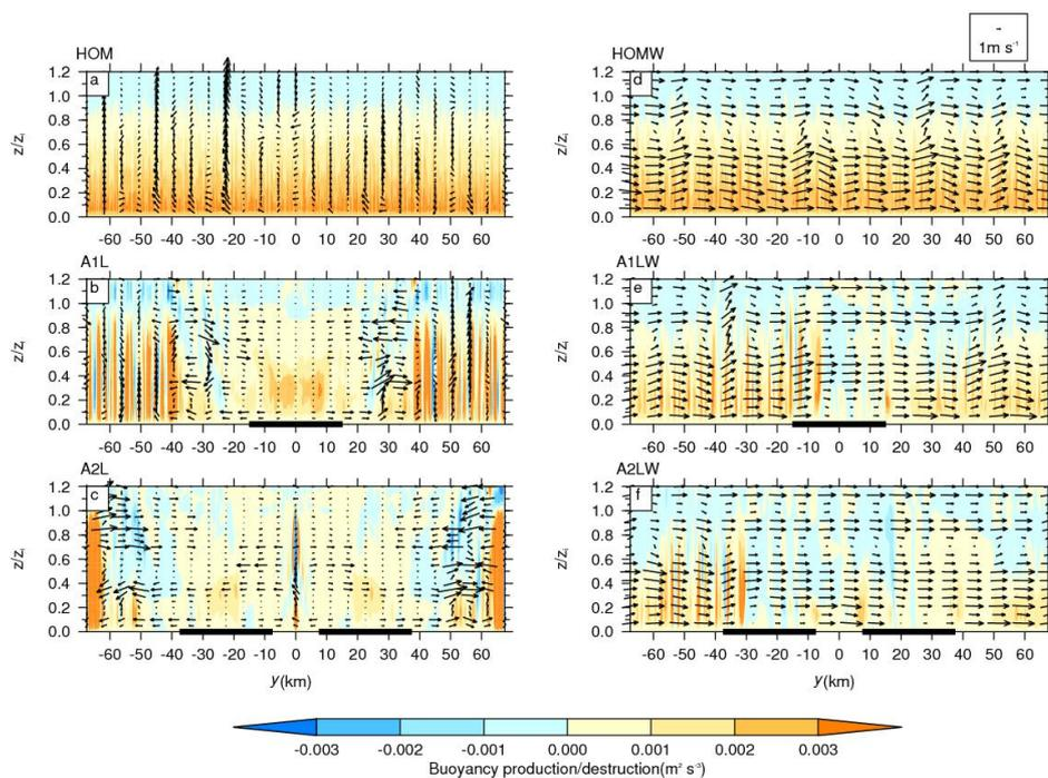
Fig. S4. The  $y$ - $z$  cross sections of the buoyancy production/destruction (contour) with superimposed wind vectors composed of  $v$  and  $w$  wind over (a, d) homogeneous and (b, e, c, f) heterogeneous surfaces with (d, e, f) and without (a, b, c) background flow. Black lines on the  $x$ -axis represent the lake patches
