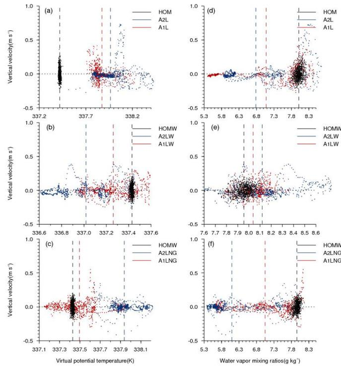
Fig. 13. The joint vertical velocities, virtual potential temperatures (a, b, c) and water vapor mixing ratios (d, e, f) at the top of the CBL for the homogeneous runs (black dot) and heterogeneous runs (red for one-lake and blue for two-lakes). The black dotted lines represent the mean vertical velocity. The black, red and blue dashed lines show the mean virtual potential temperatures and water vapor mixing ratios for the homogeneous, one-lake and two lakes runs, respectively.
