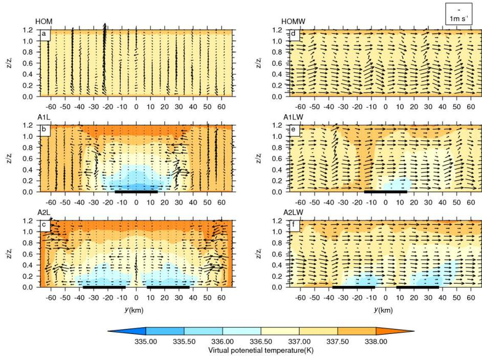
Fig. S5. The  $y$ - $z$  cross sections of the virtual potential temperature (contour) with superimposed wind vectors composed of  $v$  and  $w$  wind over (a, d) homogeneous and (b, e, c, f) heterogeneous surfaces with (d, e, f) and without (a, b, c) background flow. Black lines on the  $x$ -axis represent the lake patches
