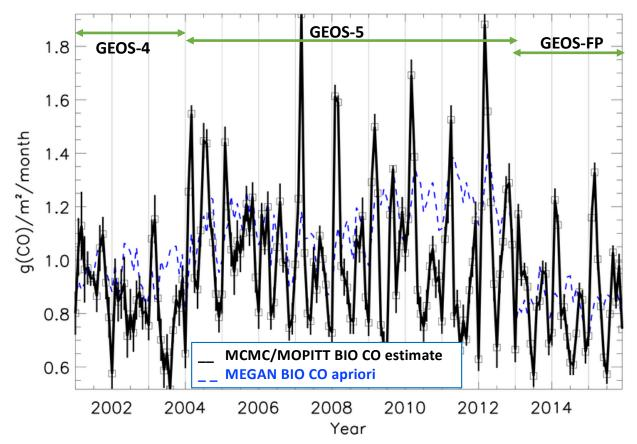
Response figure 2. Timeseries of apriori (dashed blue) and estimated CO flux (solid black, with error bars) for the <u>Equatorial Africa region</u>. Green arrows indicate the different time periods for the GEOS-4, GEOS-5 and GEOS-FP meteorological fields used to calculate the apriori with the MEGAN model and for the inverse analysis for total CO flux.
