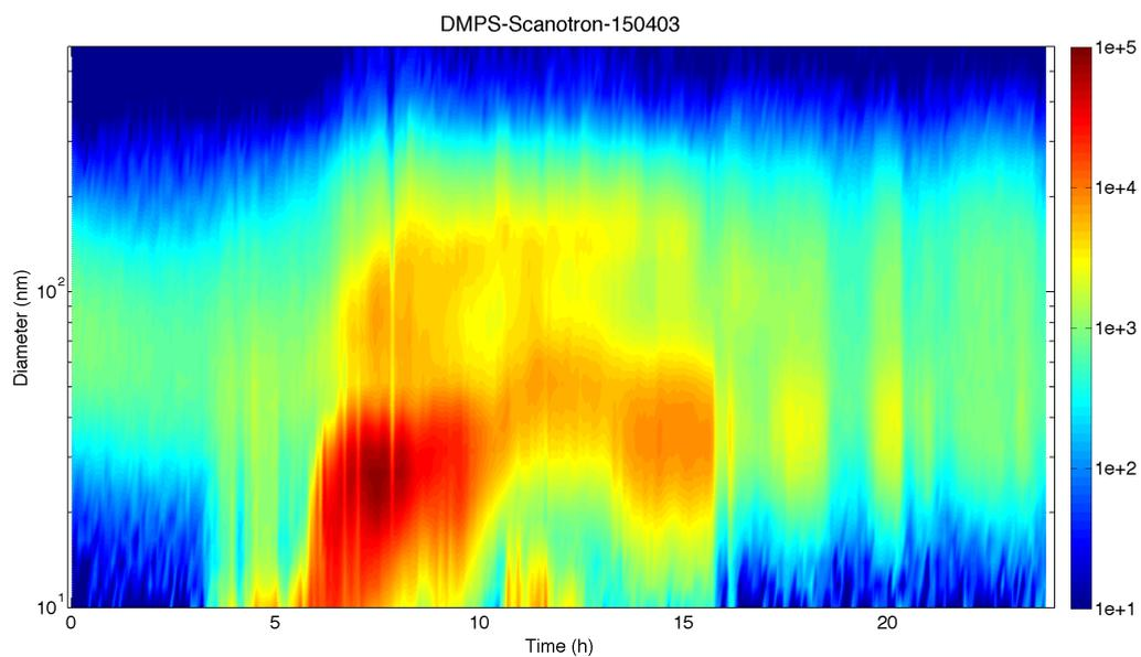
**Figure 14.** Daily variation of the aerosol size distribution (10-550 nm) observed on the 3<sup>rd</sup> of April 2015. The aerosol concentration ( $dN/d\text{Log}D_p$ ) is illustrated with the colour bar, time is on the x axis (UTC) and aerosol diameter is on the y axis.
