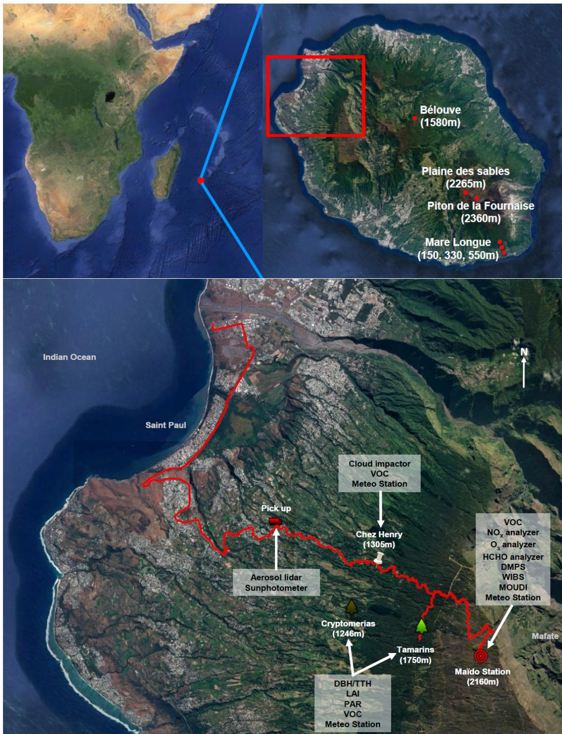
**Figure 1.** Overview maps showing the location of La Réunion as well as of the FARCE campaign sites. Altitude and deployed instruments are given for each measurement site. The red line is the pick up track on the 2<sup>nd</sup> of April 2015 (given as an example).
