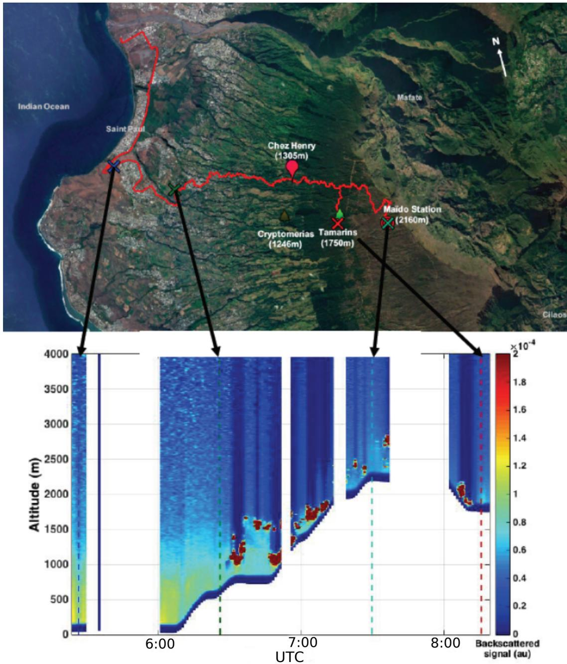
**Figure 12.** (top panel) Map showing the track of the pick up carrying the mobile aerosol lidar from Saint Paul up to the Mado station on the 2<sup>nd</sup> of April 2015. Campaign sites are shown similarly to Figure 1. (bottom panel) Lidar backscattered signals along the lidar track. Colored crosses (top panel) and dotted lines (bottom panel) show the location of the lidar corresponding to the extinction profiles shown on Figure 13.
