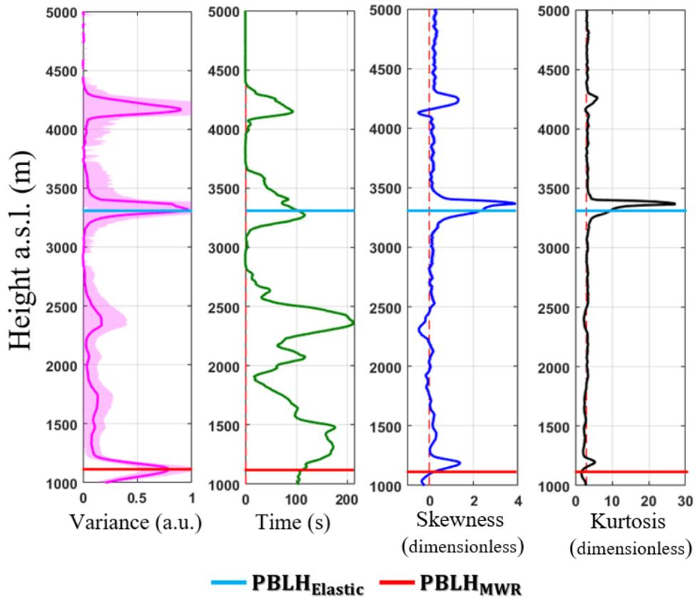
Figure 15 - Statistical moments obtained from elastic lidar data at 11 to 12 UTC - 08 July 2016. From left to right: variance [ $\sigma_{RCS'}^2$ ], integral time scale [ $\tau_{RCS'}$ ], skewness [ $S_{RCS'}$ ] and kurtosis [ $K_{RCS'}$ ].
