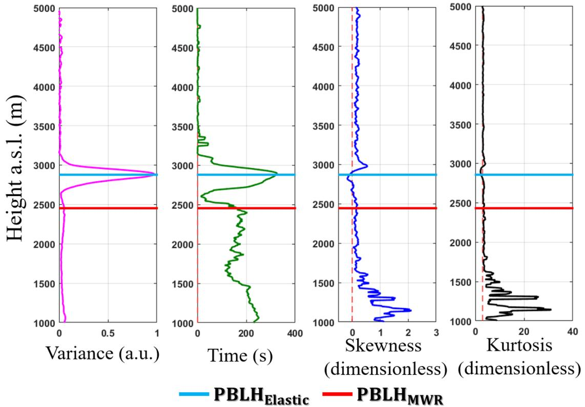
Supplementary Material - Figure 6 - Statistical moments obtained from elastic lidar data at 15 to 16 UTC - 19 May 2016. From left to right: variance [ $\sigma_{RCS'}^2$ ], integral time scale [ $\tau_{RCS'}$ ], skewness [ $S_{RCS'}$ ] and kurtosis [ $K_{RCS'}$ ].
