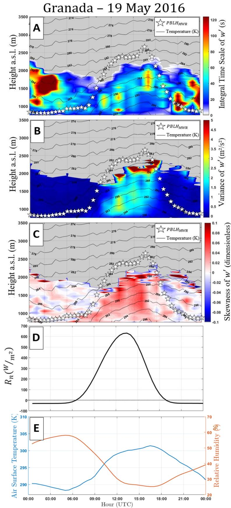
Figure 8 – A – integral time scale  $[\tau_{wv}]$ , B – variance  $[\sigma_{wv}^2]$ , C – skewness  $[S_{wv}]$ , D – net radiation  $[R_n]$ , E – Air surface temperature [blue line] and surface relative humidity  $[RH]$  – orange line]. In A, B and C black lines and white stars represent air temperature and  $PBLH_{MWR}$ , respectively.
