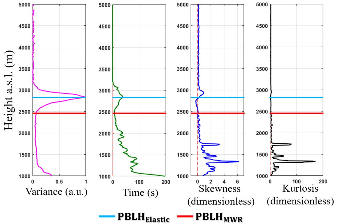
Supplementary Material - Figure 5 - Statistical moments obtained from elastic lidar data at 14 to 15 UTC - 19 May 2016. From left to right: variance [ $\sigma_{RCS'}^2$ ], integral time scale [ $\tau_{RCS'}$ ], skewness [ $S_{RCS'}$ ] and kurtosis [ $K_{RCS'}$ ].
