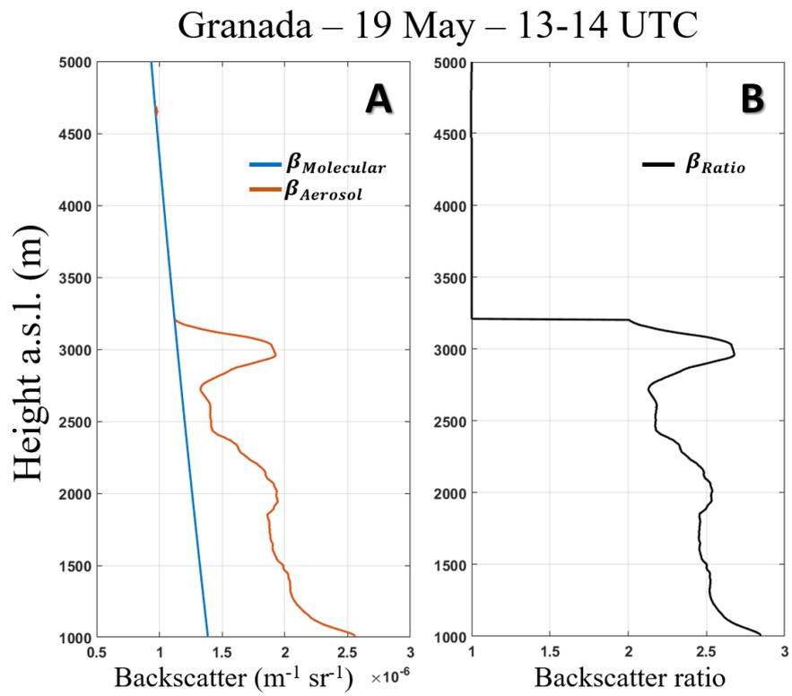
Figure 10 – (A)  $\beta_{Molecular}$  (blue line) and  $\beta_{Aerosol}$  (orange line). (B)  $\beta_{Ratio}$  (black line). All profiles were obtained from the 532 nm lidar signal
