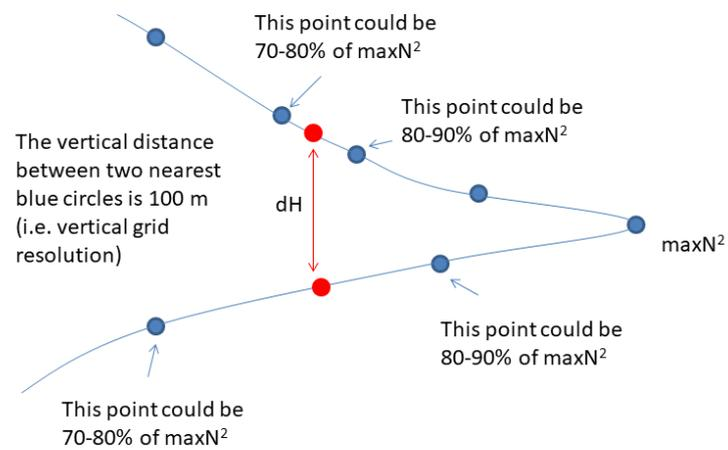
**Fig. 1.** The diagram of the algorithm to calculate  $dH$  from the  $N^2$  profile.
