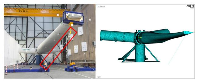
10 Figure 1: Pitch bearing test rig at Fraunhofer IWES and corresponding FE model.
