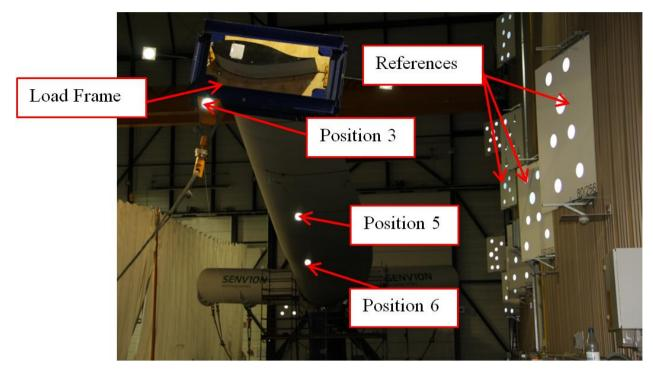
Figure 2: Optical position measurement.
