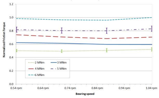
Measured friction torque at different speeds and loads
