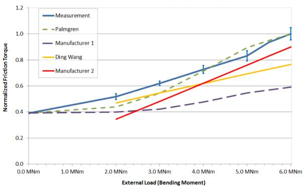
Friction torque at different loads (averaged over speeds)
