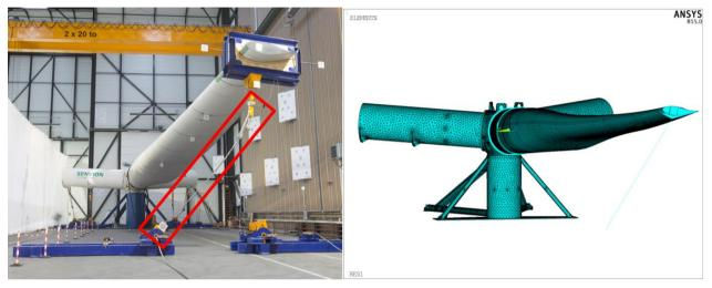
Figure 1: Pitch bearing test rig at Fraunhofer IWES and corresponding FE model.
