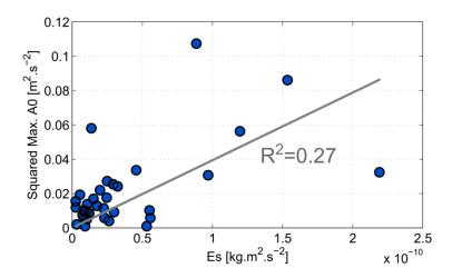
**Figure 1:** Squared maximum amplitude A0 as a function of the energy of the seismic signal generated at each impact
