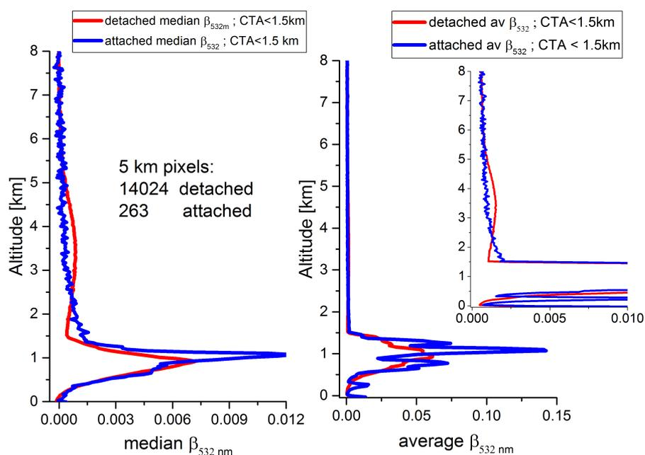
Figure 3.R1. Median (a) and averaged (b) backscatter profiles ( $\text{km}^{-1}\text{sr}^{-1}$ ) for aerosol layer detached from the cloud layer (red) and aerosols attached to the top of the cloud (blue), for the period May-October from 2006 to 2010, over the South Atlantic Ocean region. The data was filtered for a cloud top altitude lower than 1.5 km.
