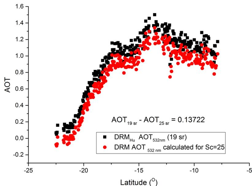
Figure 2.R1 presents the above-cloud AOT at 532 nm for  $DRM_{Hu}$  (19 sr) and DRM at 25 sr in function of latitude for 4 August 2008, for a case of biomass-burning off-coast of Namibia.
