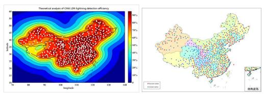
Fig.1 Left is theoretical distribution map of detection efficiency, right is CMA LDN station distribution plan map (blue point is existed station, red point is planned station, total station number is 599).
