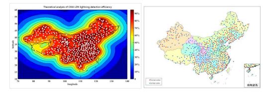
Fig.1 Left is theoretical distribution map of detection efficiency, right is CMA LDN station
