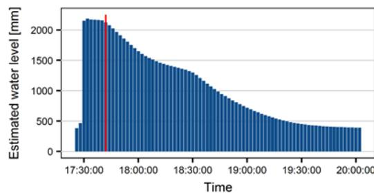
**Figure 5:** Signs of leakage visible in the water level at manhole m2 (sensor m2\_h\_p\_endress\_minilog). The pipe network should not be able to drain but over the course of two hours, starting at the red line, the water level in manhole m2 falls by around 1.7 meters.
