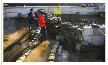
Figure 2: View from camera CAM1 in which a bicycle is visible in the flood water behind the dam. Deep learning could make it possible to automatically estimate the water level from such an image. An ultrasonic sensor above the water and a pressure sensor in manhole m1 provide water level data.
