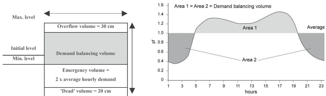
Fig. 1. (a) Required tank volume; (b) Demand balancing volume (adapted from Trifunović, 2006)
